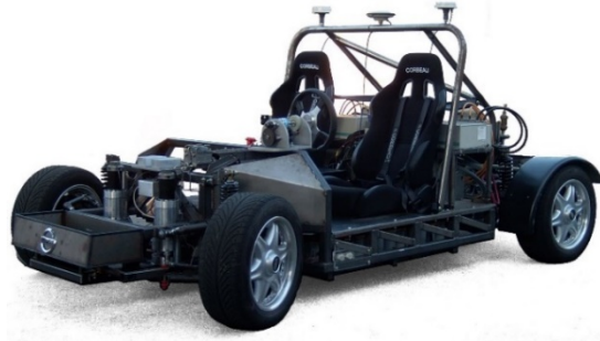
Figure 6: P1 steer and drive by wire test vehicle
