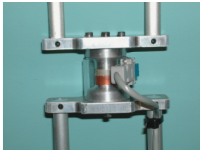
Figure 4: Complete left crutch with load cell built into it
