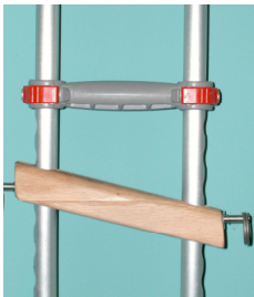
Figure 3: Load cell incorporated into left crutch
